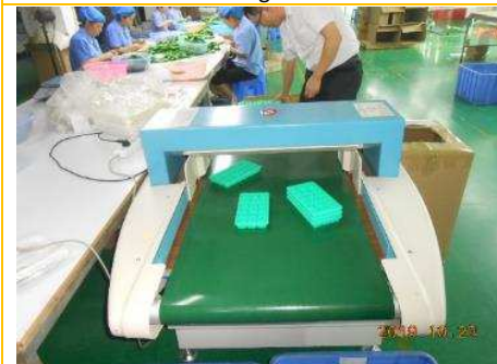
metal detection for finished product
